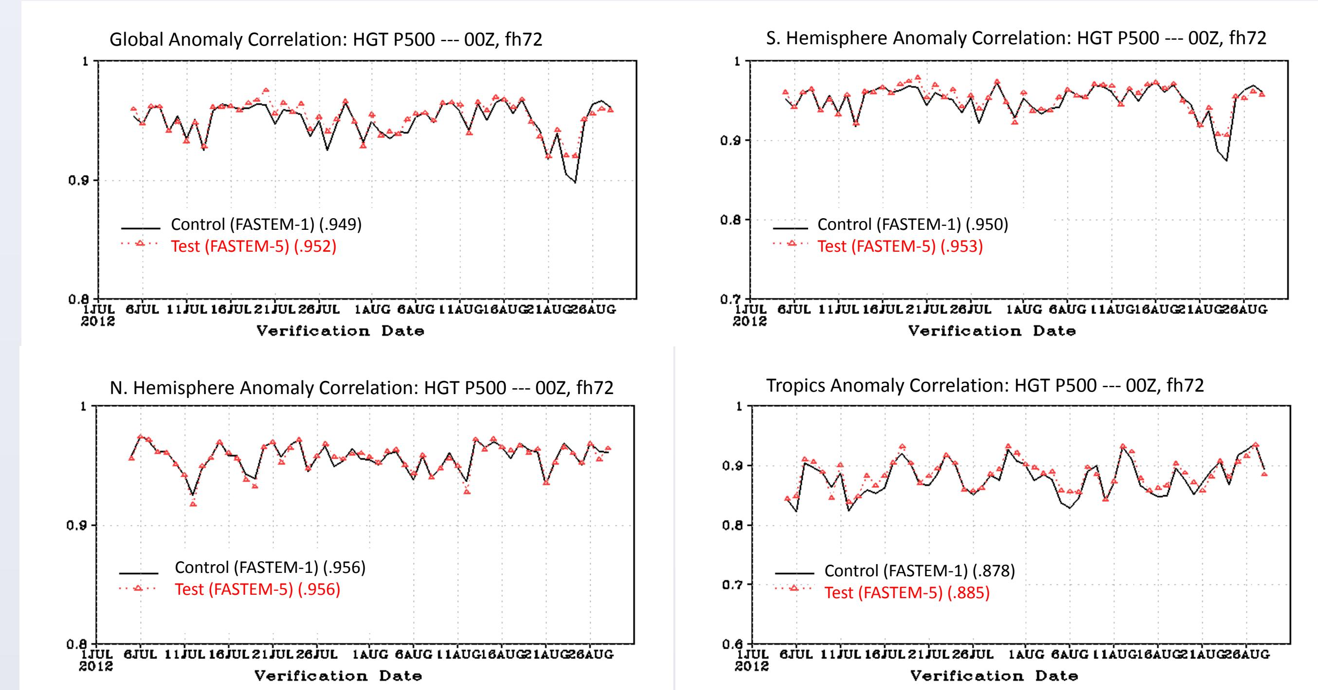
Figure 2 Three day forecast anomaly correlation (AC) scores for a GFS 3dvar T254 parallel experiment. The control AC scores are in black and the test AC scores are in red. The forecast anomaly correlation scores shown are with respect to their own analyses.
